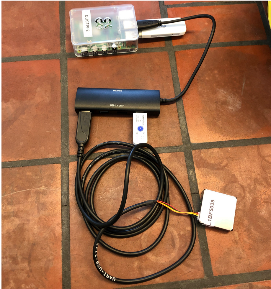
Figure 3.2: Sensor system and raspberry pi, where one sensor is connected marked 1BF5039.
