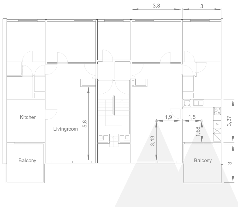
Figure 2.25 Illustration of the points of view and window viewing angles used in the view study
