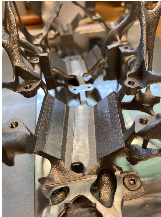
Figure 28: The machined v-groove
