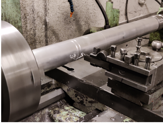
(a) Turning new mast stub on a lathe
