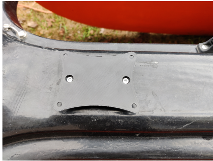
(c) Mount attached to sailboat (d) IMU mounted on sail boat
