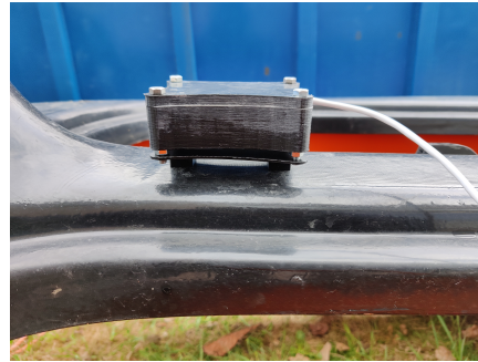
(c) Mount attached to sailboat (d) IMU mounted on sail boat
