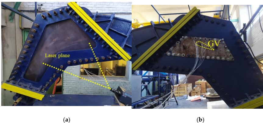
Figure 6. The three-GV test setup for experimental validation: (a) Experimental set up which shows the test section in the lab ; (b) Locations of holes for tapping the value of pressure at GV.
