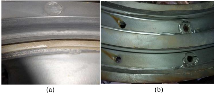
Figure 4. Erosion at upper labyrinths (a) Towards the rotating side and (b) Towards the stationary side [Taken from Paper 3 ].
