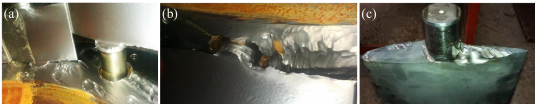
Figure 1. Erosion due to secondary flows at the clearance gap of GVs (a) Towards bottom facing plate and (b) Towards upper facing plate & (c) Eroded GV towards the bottom end [Taken from Paper B ].
