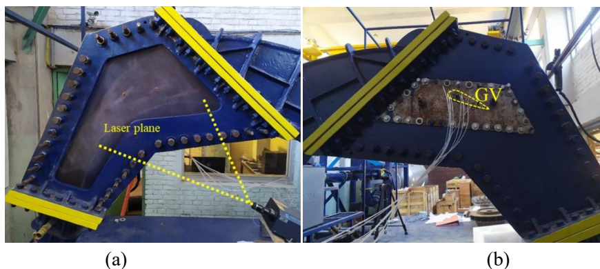
Figure 6. The three-GV test setup for experimental validation: (a) Experimental set up which shows the test section in the lab ; (b) Locations of holes for tapping the value of pressure at GV [Taken from Paper 3 ].
