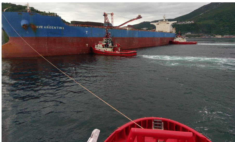
Figure 1.3: Manual tugboat assisted docking of a bulk carrier in Narvik. Photo: R. Kristiansen
