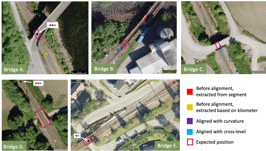
Figure 5.13.: Extracted positions of the bridge objects based on the superstructure record before and after alignment, compared to visually expected position of the bridge objects. Satellite images extracted from Gule Sider [2].
