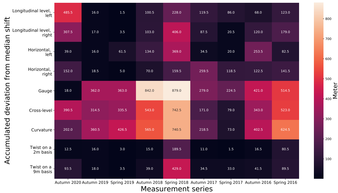
Figure 4.7.: Heat map displaying deviation in found shift for each measurement channel when compared to the median shift. Each measurement series is evaluated separately.
