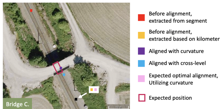
Figure 5.16.: Extracted coordinates, from the spring 2020 measurement recording, for bridge C based on the manual alignment between the superstructure record and measurement series. Observe how the position extracted from the measurement vehicle after assumed optimal alignment is outside the expected position range for the bridge object. Satellite image extracted from Gule Sider [2].
