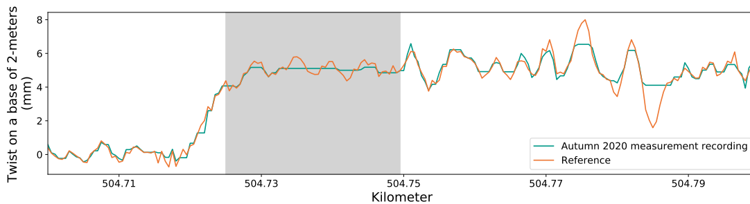
(b) Track measurements recorded autumn 2020 compared to the reference, further aligned with DTW.
