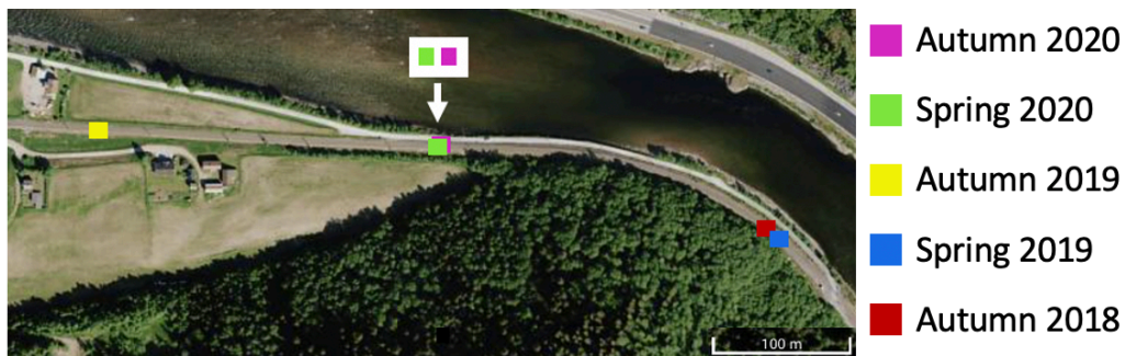
Figure 4.9.: Deviations in absolute position for a specific measurement, retrieved from the different measurement recordings equipped with GPS, despite relative alignment.
