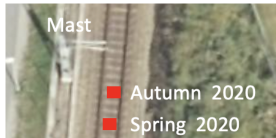
Figure 4.10.: Satellite image of mast EH-MAS-023826 compared to the extracted GPS location of the same mast from recorded data spring and autumn 2020. Image obtained from Gule Sider [2]
