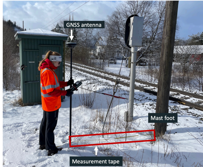
Figure 4.12.: Field measurement at mast EH-MAS-023281. Measuring coordinates at position 2 with the GNSS antenna and the distance from the position to the mast foot utilizing measurement tape.
