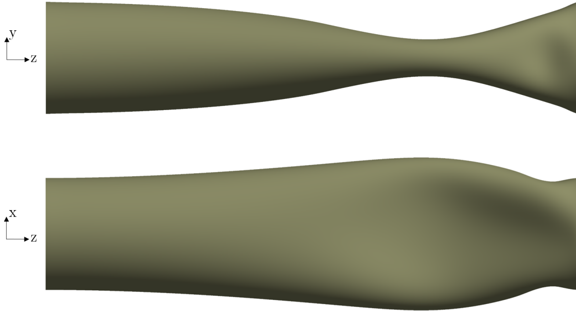
Figure 5.3: Deformation of the flexible part of the tube from two views. Images used courtesy of ANSYS, Inc.
