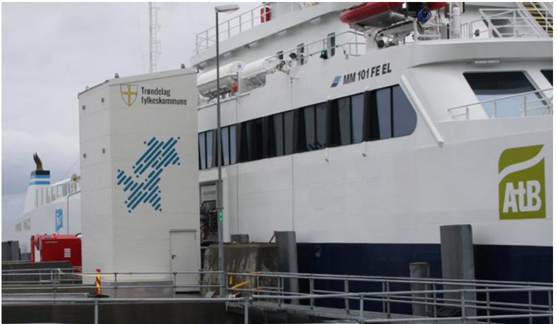
MF Lagatun docking by the charging station at Flakk. Photo credits: Karl-Henrik Linder
