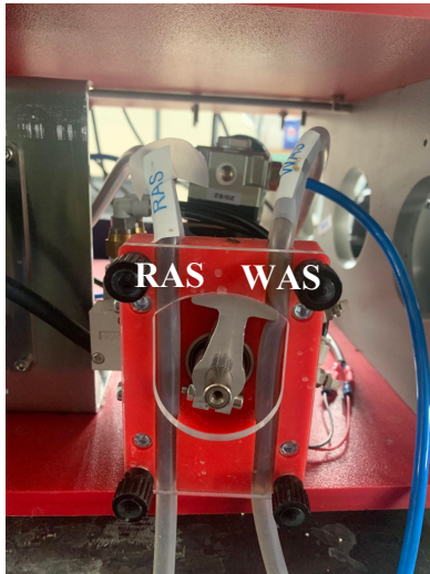
Figure 12: A picture of the RAS and WAS valve for the lab - scaled pilot.
