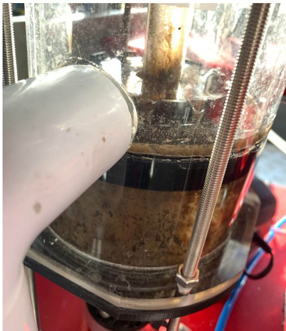
Figure 19: A close up of the settler in Stage 2.
