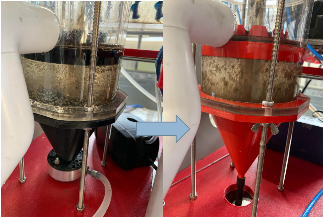
Figure 22: The picture shows the design of the old and new settling tank.
