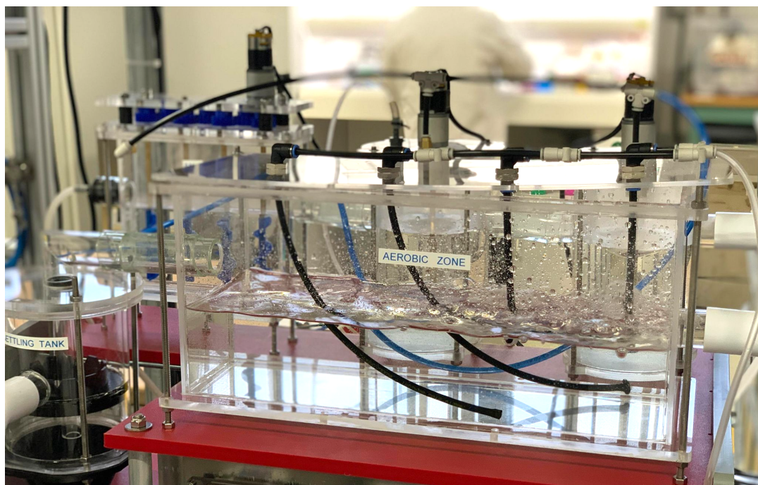
Figure 10: The picture shows the aerobic reactor. The aeration system shown in this picture has not been used during the experiment period.
