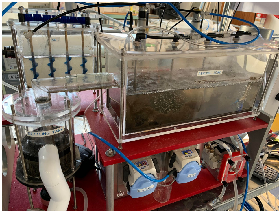
Figure 15: The picture shows how the pilot looked in Stage 1 after left to operate by its own. All chambers are diluted and most of the sludge has settled in the aerobic reactor.
