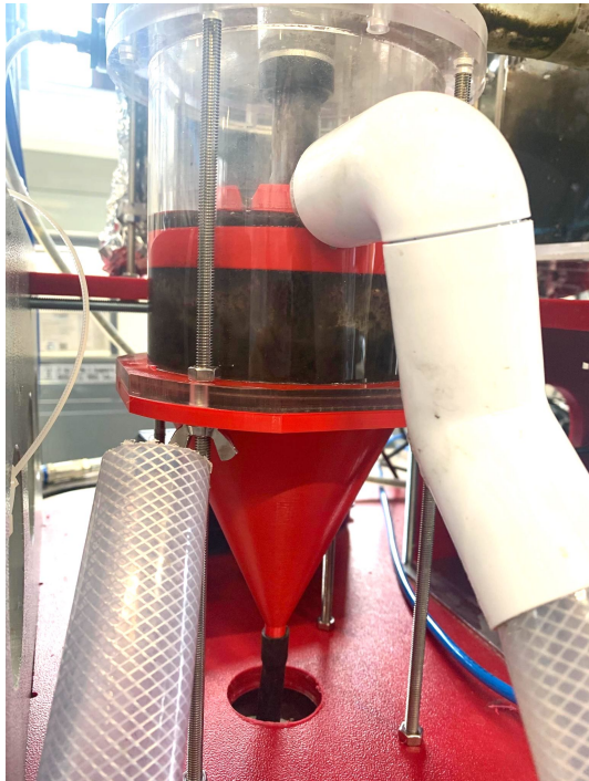
Figure 26: Picture of the pilot settling tank at 25.04.22. Sludge have started to accumulate.
