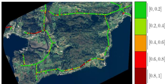
Figure 5 – Heatmap using a Tree Density Index to indicate high and low exposition of power lines to trees.
