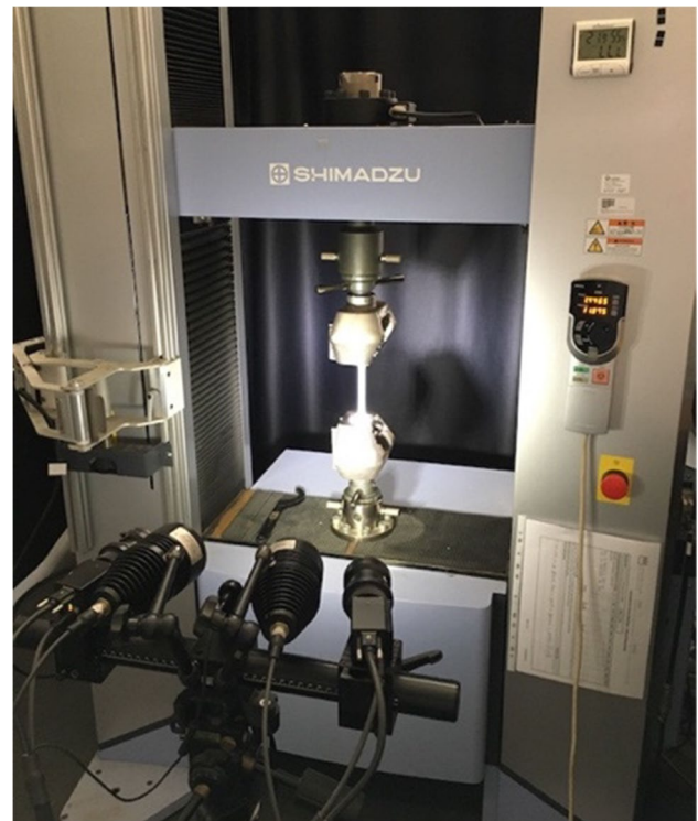
Fig. 2 Shimadzu AG-X100kN and DIC (GOM)
