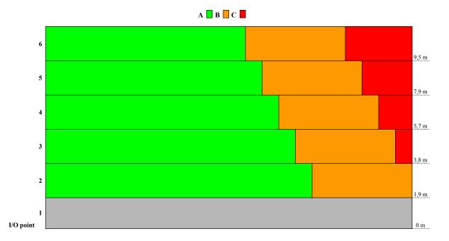
Figure 4.19: The zones A, B and C for the relevant shelves for reshuffling in the full pallet area. The figure shows one arbitrary rack as seen from the side with the corresponding zones (the zones are similar for all relevant racks). The heights in the bottom of each shelf are shown to the right of the figure. Shelf number 1 is shown in gray because it is not relevant for the analyses in this area.
