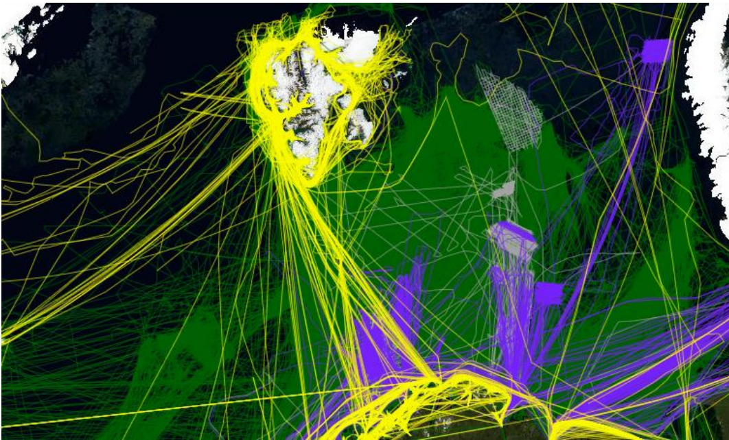
Figure 2 - AIS data from the year 2014 shows the extensive traffic in the Barents-sea. Green: fishing activity. Yellow: passenger ships. Purple/grey: offshore activity. (havbase.no, 2014)
