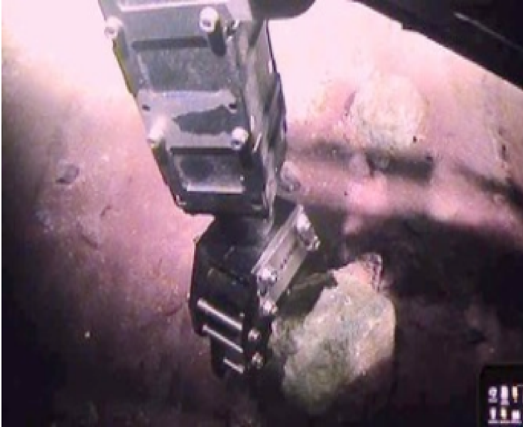
Figure 28: Sea-bed surface grab sampling by HyBIS RUV at TAG field area.
