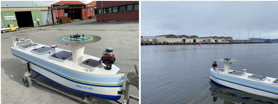
Figure 3.5: Helipad mounted on ReVolt vessel for drytesting and seatrials.
