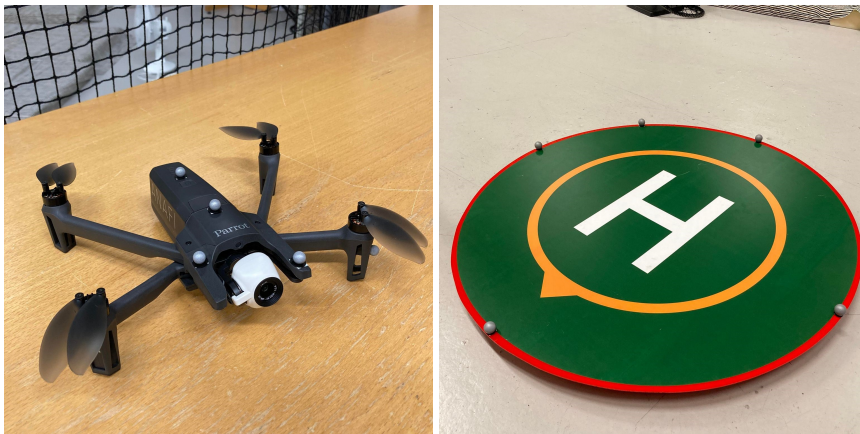
Figure 3.7: Anafi and helipad with attached optical markers.
