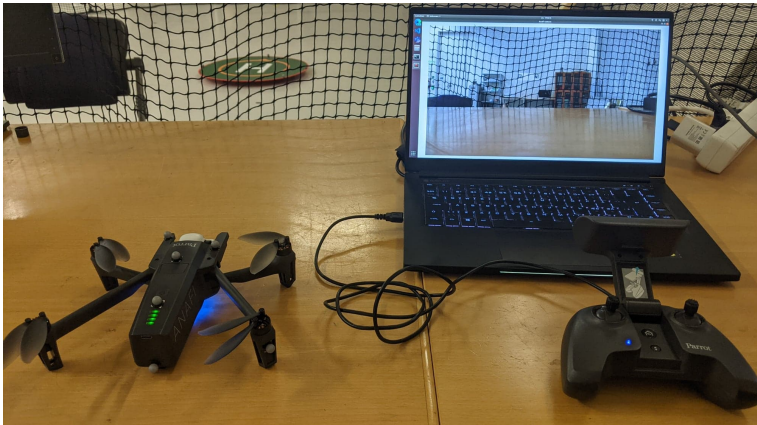
Figure 3.2: Image showing the Anafi connected to the computer using the Skycontroller 3 as a relay.
