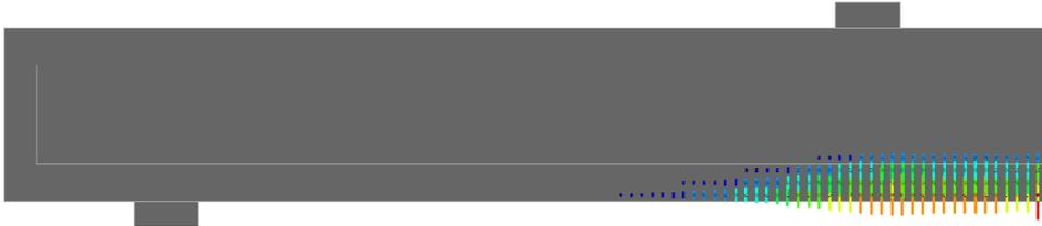
*Figure 4.26 – Crack strain plot before the crack localizes for the damage based shear retention model in beam S1D18a108*
