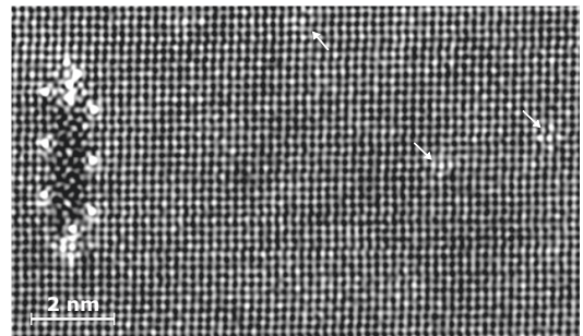
Fig. 4. HAADF-STEM image of NA20hn showing structural units of GPB zones indicated by white arrows, in addition to one example of the lath shaped L phase on the left hand side.
