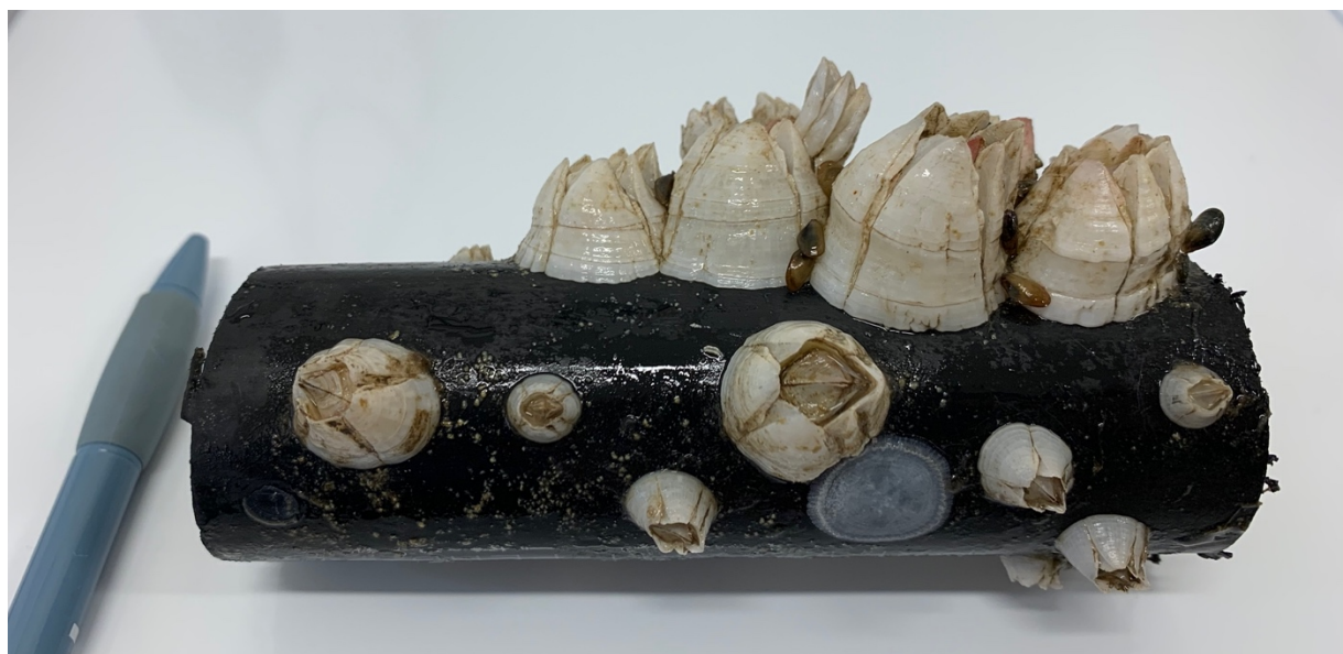
Figure 7 PVC pipe showing large 22-month-old barnacles on top of the pipe. Pen for size reference. The "normal" sized (10-13 mm in length) barnacles in lower right corner are one year younger than the large ones.
