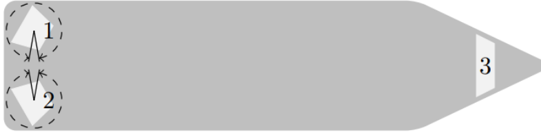
Figure 2.2: Thruster configuration for the marine vessel. Illustration from [29]
