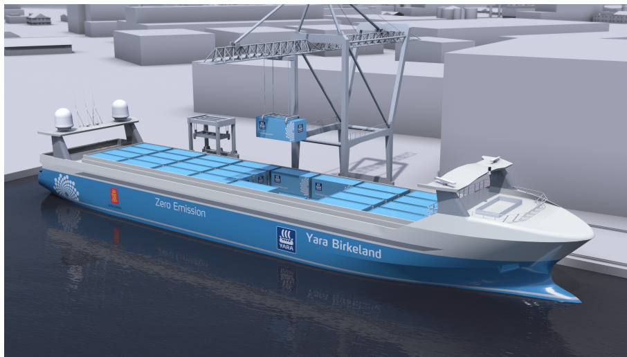
Figure 1: Yara Birkeland, Kongsberg Maritime’s autonomous container ship project (Kongsberg Maritime 2022). Image courtesy of Yara International ASA.
