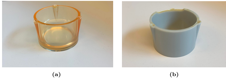
Figure 4.2: Cast cups: (a) Epoxy cup without silica filler; (b) Epoxy cup with silica filler.
