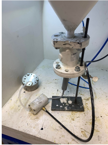
Figure B.1: Setup for the casting of epoxy with silica cup.
