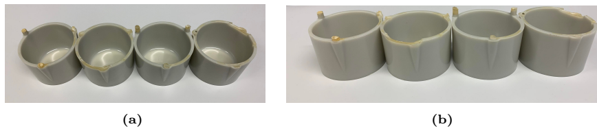
Figure C.10: The epoxy with silica flour cups made in the second casting with silica flour.
