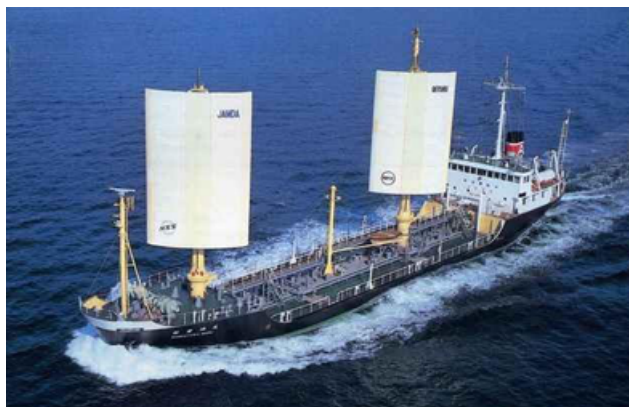
Figure 2.4: Shin-Aitoku Maru fitted with wingsails
