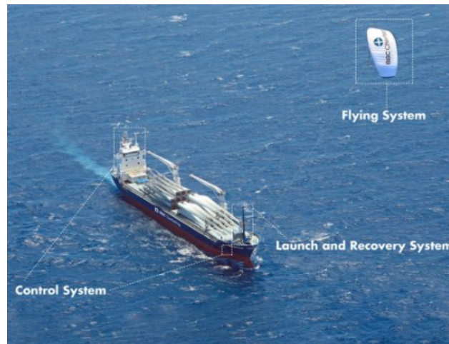
Figure 2.5: BBC Skysails fitted with towing kite
