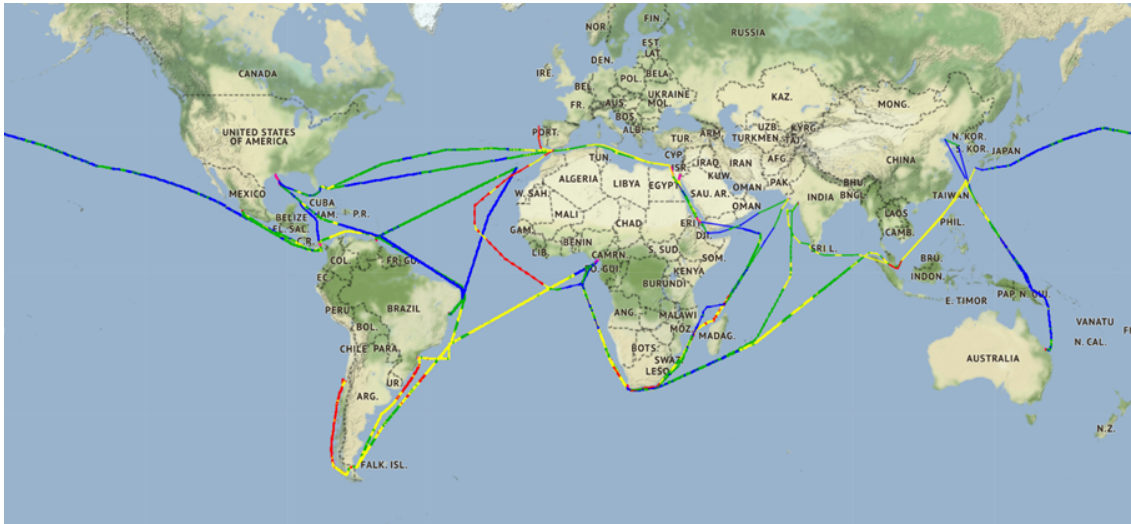
Figure 7.1: Vessel routes; >18 knots (blue), 16-18 knots (green), 14-16 knots (yellow), 10-14 knots (red), <10 knots (pink)
