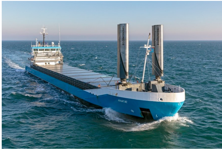
Figure 2.6: General cargo vessel Ankie fitted with two suction wings
