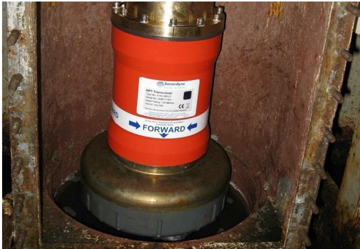
Figur 86: Through hull-montert transceiver
