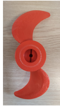
(b) 3D printed version of original otter propeller
