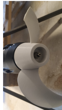
(b) 3D printed version of the broken propeller
