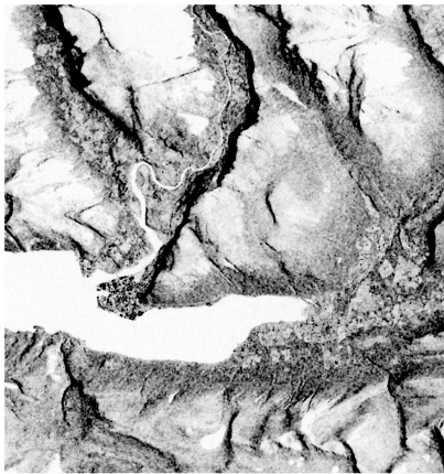
(e) Step 4: Speckle filtering with Frost-filter. Plot of Sigma0_VH band.
