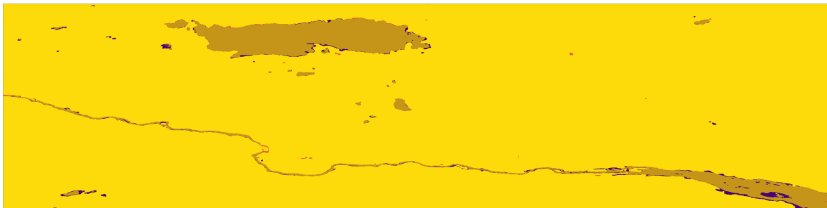
Figure 4.25: Comparison of the two Bismo images predicted by U-Net. The darkest violet colored areas was only detected in the October image, while the orange colored areas was only detected in the September image.
