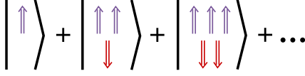
FIG. 1. Representation of a spin-up antiferromagnetic squeezed magnon [51]. The squeezed excitation is a coherent superposition of states with N + 1 spin-up and N spin-down magnons. Each of the constituent states possesses a unit net spin, but varies in its spin content on each sublattice, thereby resulting in strong quantum fluctuations.
