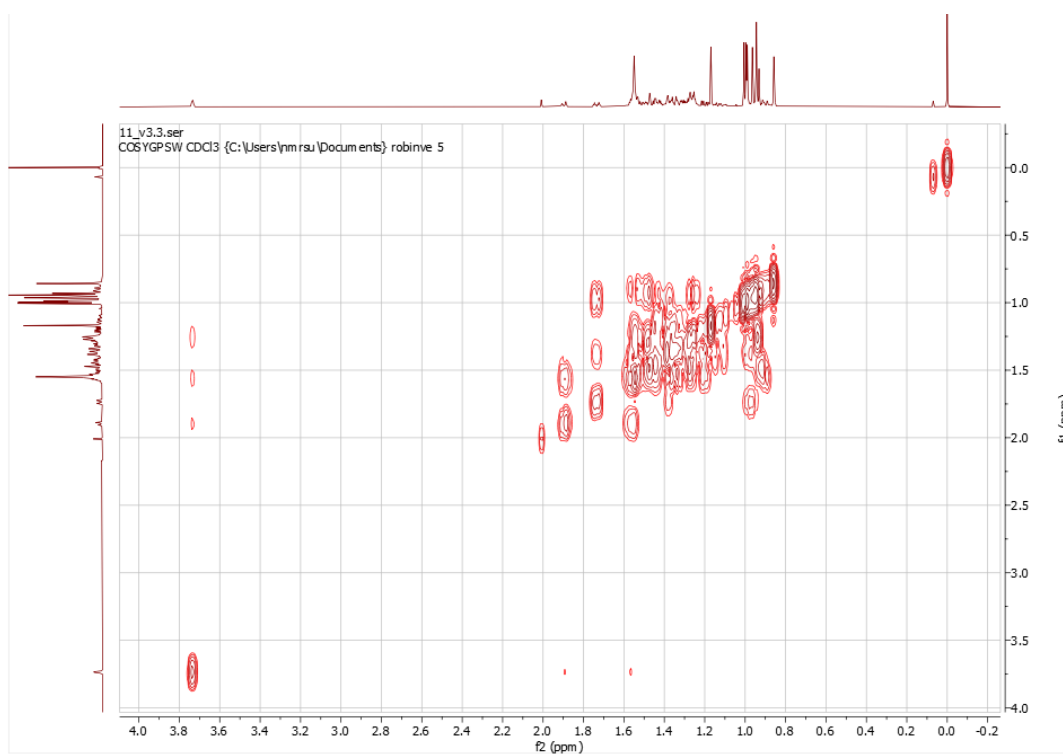
Figure A.11.8: COSY spectrum obtained for Sa-11 with pulse sequence cosygpppqf and 2 scans.
