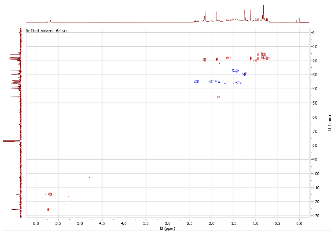
Figure A.6.3: Edited HSQC spectrum of Sa-6 obtained with pulse sequence hsqcedetgpsisp2.3 and 8 scans.
