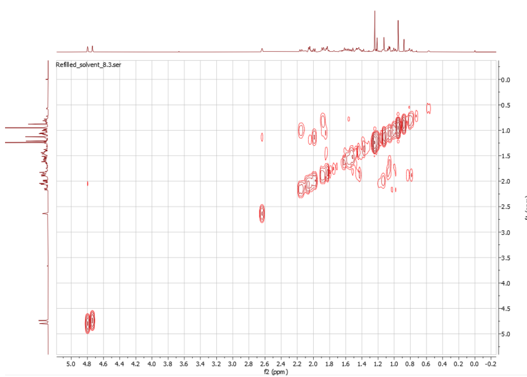
Figure A.8.8: COSY spectrum of Sa-8 obtained with pulse sequence cosygpppqf and 4 scans.
