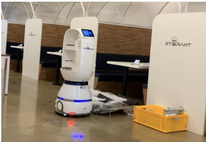
Figure 15: Delivery-Robot versus Bubble Wrapper: "its wheels caught in a piece of bubble wrapper".
