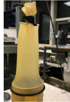
Figure 5.19: Picture of conducted membrane stiffness in extension.
