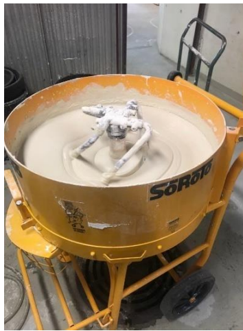
Figure 3. 2: Mixing of kaolin and water using a mortar machine.
