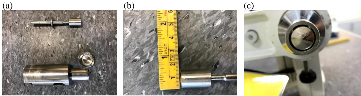
Figure 3. 6: (a) rotor and outer cylinder, (b) diameter of rotor, (c) R_0/R_i , gap of 1.1
