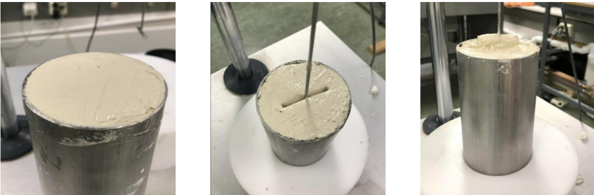
Figure 3. 12: Shows Kaolin clay at 62% water content, from left: before cycling, middle: during cycling, right: after cycling.
