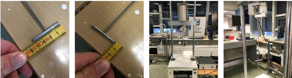
Figure 3. 8: T-bar cylinder dimensions and apparatus
