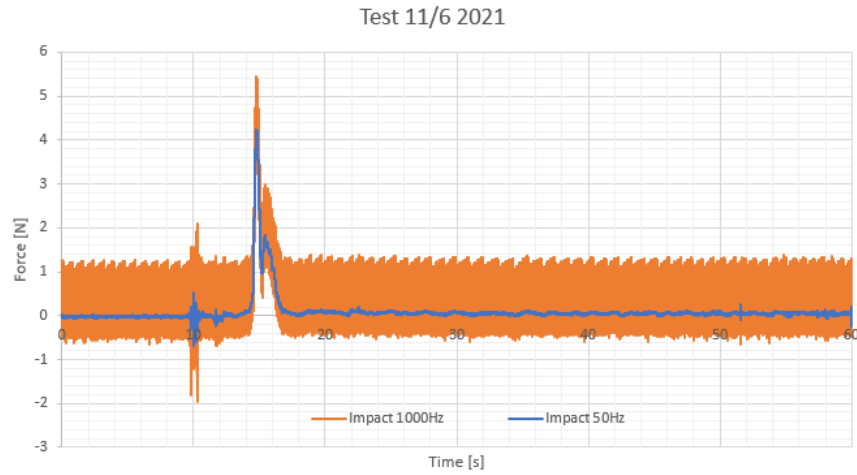
Figure 4. 7: Impact force measurements, 1000Hz represents the entire sampling domain and 50Hz represents data processed results. This test represents test 15 in Table 4. 1.
