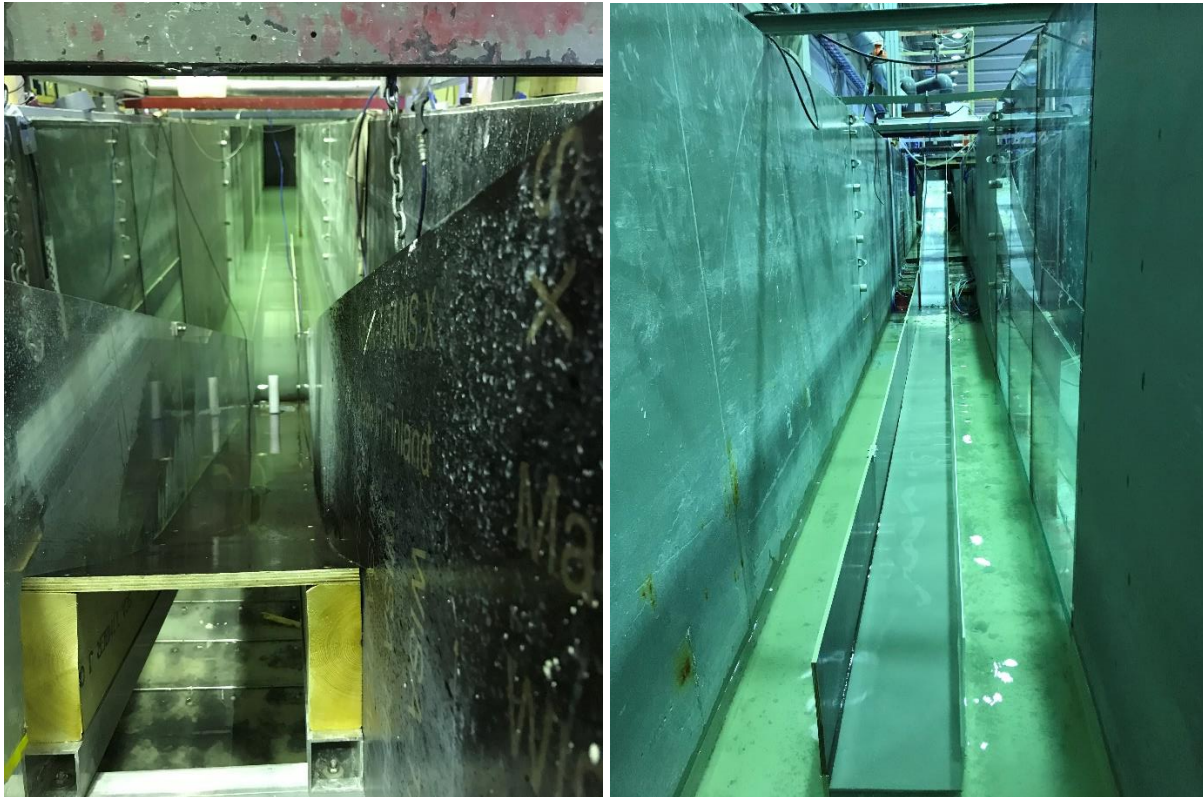
Figure 4. 1: Empty model flume at NTNU Hydrolab. Left picture shows the impact pile placed in the middle of the flume, approximately 2.75m from the slide initiating area.
