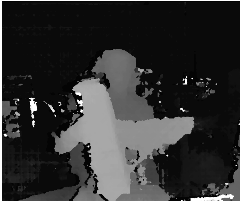
Figure 4.2: A complete disparity map calculated from someone sitting in front of the camera holding two objects at different distances from the cameras. Notice the noise as completely black and white areas in the disparity map.
