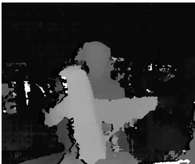
Figure 2.6: Disparity map shown as gray-scale image. Bright features are close to the cameras, and dark features are further away. The black areas represent features as far away from the camera that correspondence is not found.
