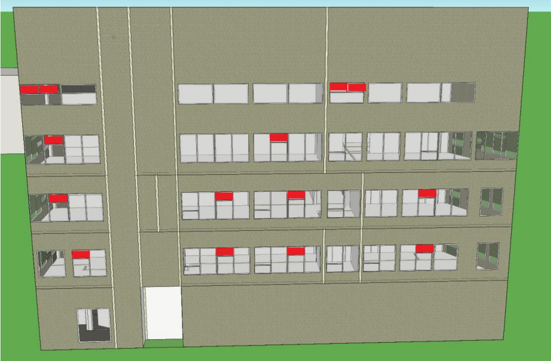
Appendix A-1: Windows with automatic control on the north façade marked in red.
