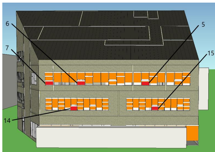
Figure 18: Points of differential pressure measurements on the south façade at the ZEB lab
