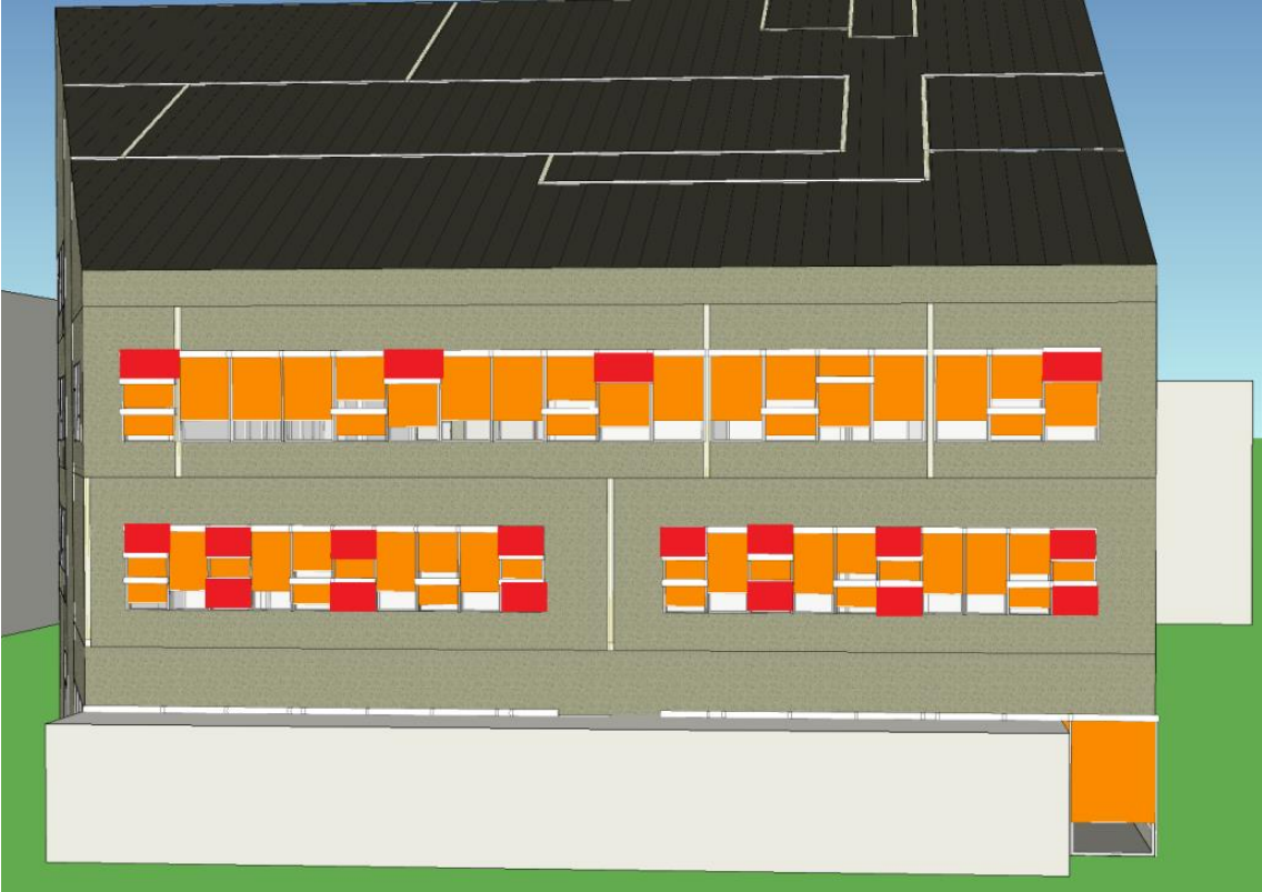
Appendix A-2: Windows with automatic control on the south façade marked in red
