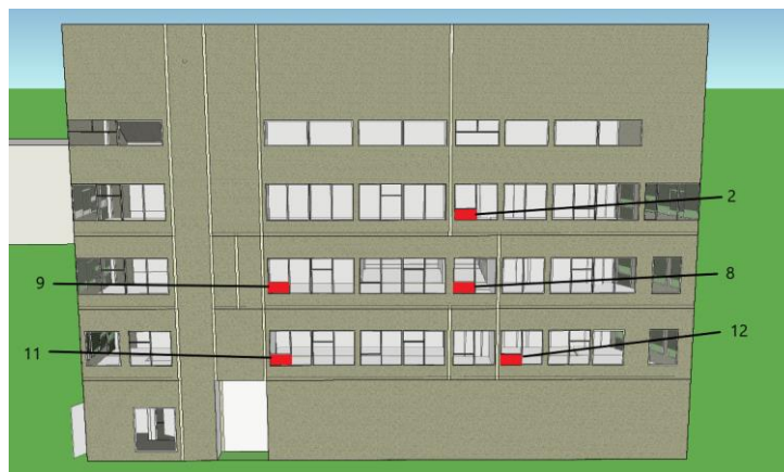
Figure 17: Points of differential pressure measurements on the north façade at the ZEB lab
