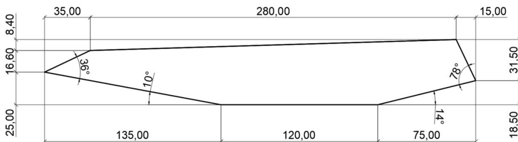
Figure 4.1: Cross-section of the upstream-box.
