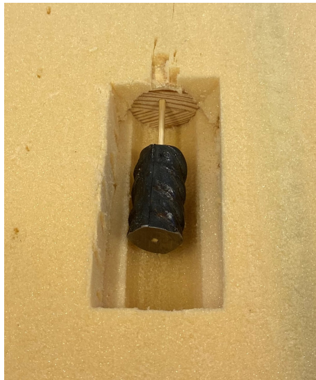
Figure 4.17: The self-made TMD
