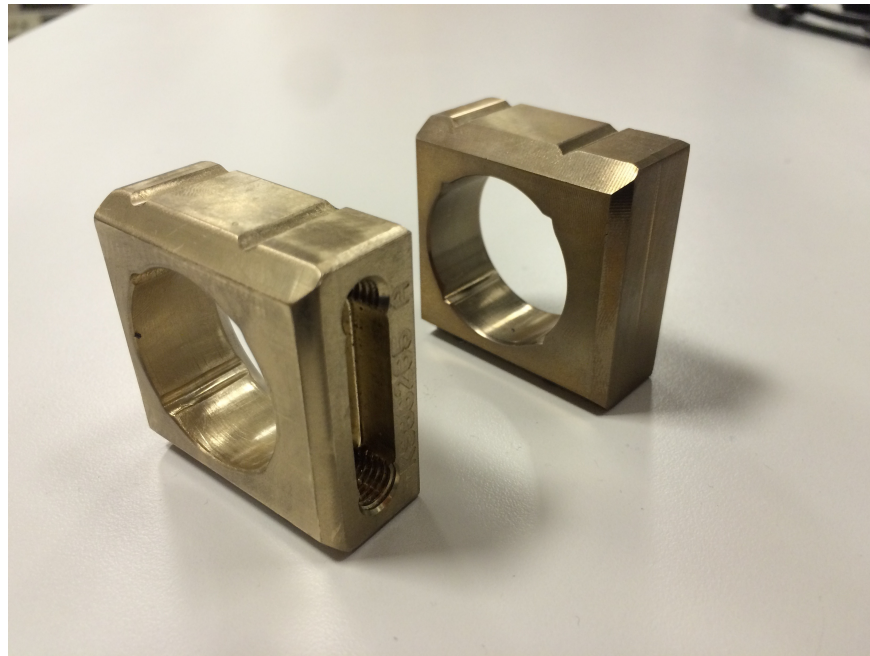
Figure 3.30: Slide bearing modification
