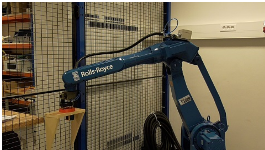
Figure 4.28: Robot picks up the thruster disc rotation tool
