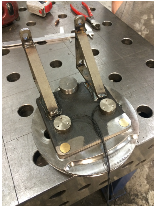
Figure 3.28: Testing fitment of gripper on the thruster disc
