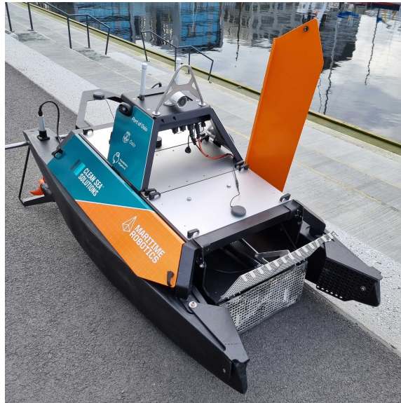
(a) The CDV1 cleaning drone seen from the front with the backplate of the collection bin pushed out.
