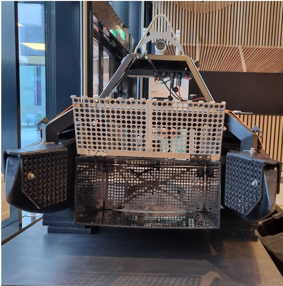
Figure 13: The CDV1 trash bin mounted between the pontoons of the USV.
