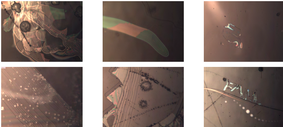
Figure 67: Irregularities and cracks observed on the mica substrate by using OM at UC Berkeley
