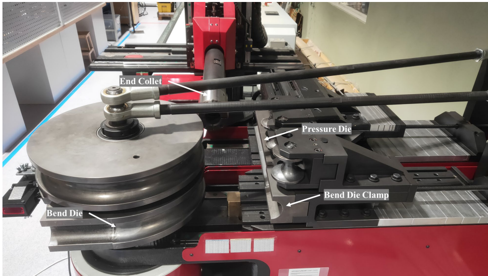
Figure 1. STAR EVO 800 Bending machine.
