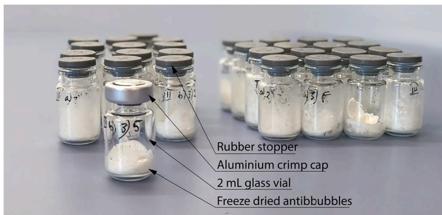
Fig. 6. Photograph of a batch of antibubbles after being lyophilized. The cake can be seen to easily detach from the vial. The imperfect appearance with lyophilised product on the vial is due to the process of filling the vials by contacting the vial surface and motion prior to dipping in liquid nitrogen.
