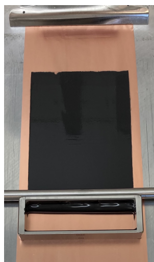
Figure 3.1: Experimental procedure of tape-casting.
