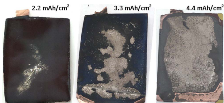
Figure 2.9: Graphite electrodes with different thicknesses and loading of 58 \mu\text{m} ( 2.2mAh/cm 2 ), 97 \mu\text{m} (3.3 mAh/cm 2 ) and 127 \mu\text{m} (4.4 mAh/cm 2 ) after cycling [58] .
