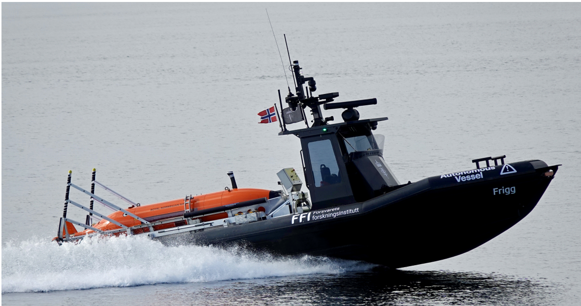
Figure 1.1: The USV, and the AUV on top of the attached LARS. Courtesy of FFI.
