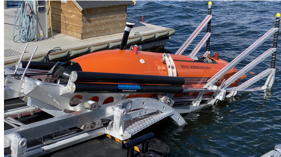
(4) The AUV is attached to the Stinger and can be lifted onto the USV
