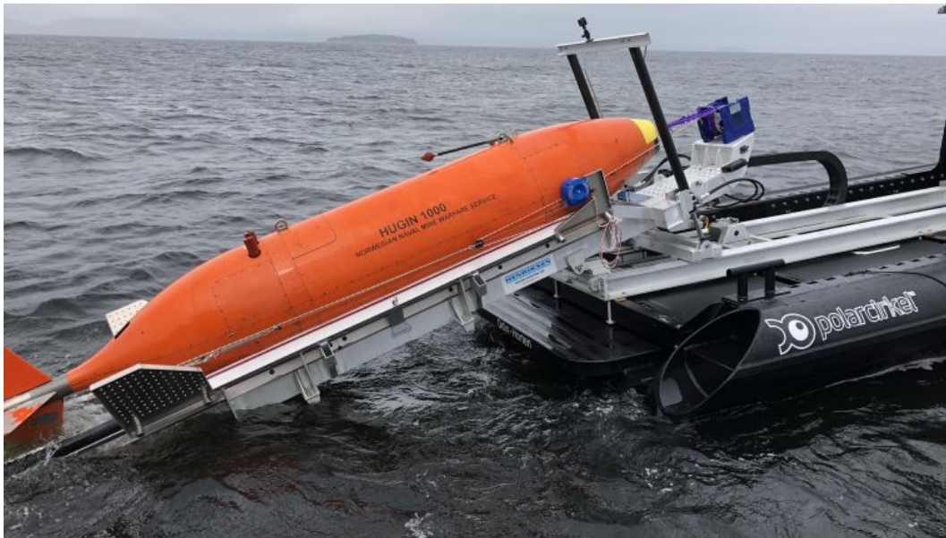
Figure 2.6: The Stinger, mounted on the USV, recovering Hugin. ©Hydro International [17].
