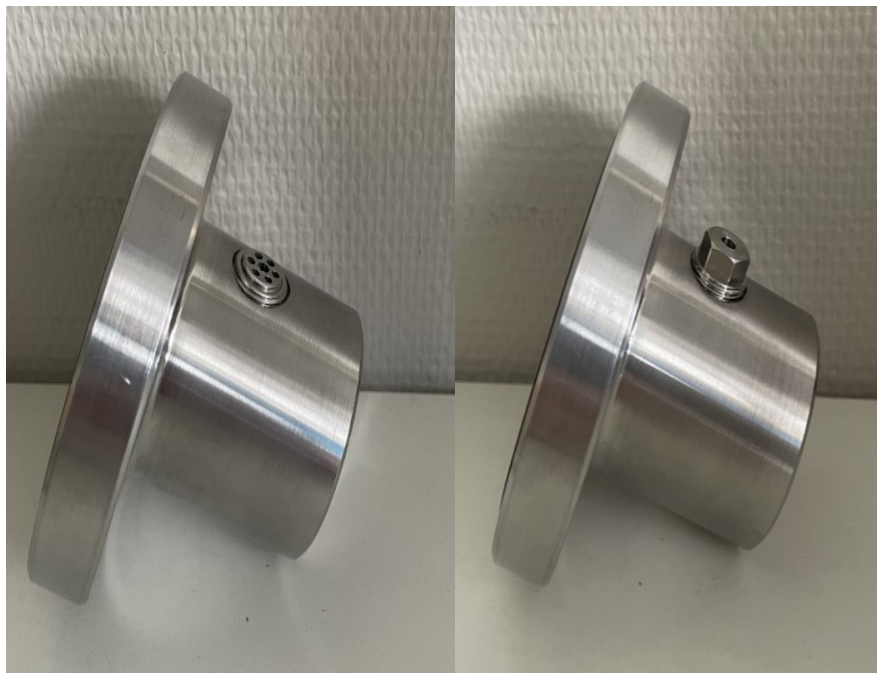
Figure 3.12: Valve holder with the injection valve ( left ) and production valve ( right )
