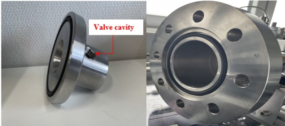
Figure 3.2: Valve holder ( right ) and the outside enclosure ( left ) that make up the pressure cell
