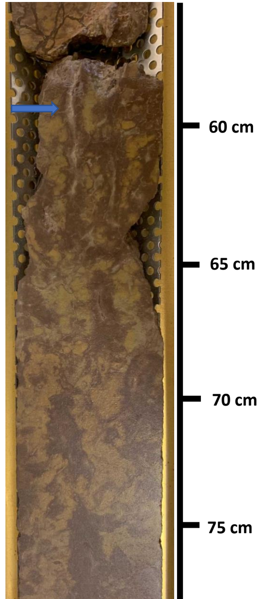
Figure 22: Core photos showing mottled claystone. (a) Red and white coloured mottled claystone. (b) Multi coloured mottled claystone, possible rootlet indicated by arrow.
