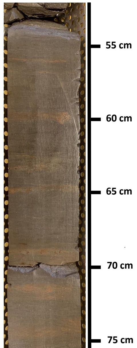
Figure 18: Core photos showing laminated mudstone. (a) Laminated mudstone with silt laminae. (b) Laminated mudstone with red pyrite or siderite laminae.
