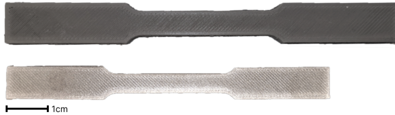
Figure 38: The green part on top and the sintered specimen on the bottom.
