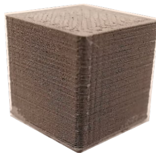
Figure 12: Printed specimen from the specialization project with dimensions of 1\text{cm} \times 1\text{cm} \times 1\text{cm}
