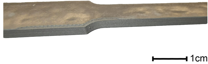
Figure 35: Some uneven first layers are observed for the tensile specimen.
