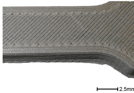
Figure 31: Gaps between strands are observed on the top layer of the tensile specimen.
