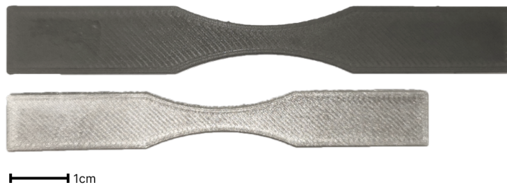
Figure 39: The green part on top and the sintered specimen on the bottom.
