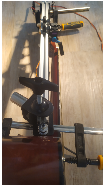
Figure 5.7: Clamps attached to hold the RoboCapo on the Guitar
