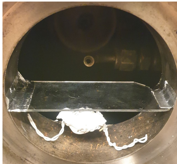
Figure 3.8: Illustration of particle placement setup. The three configurations were either static in the basket, on the glass shelf or injected through the pipe
