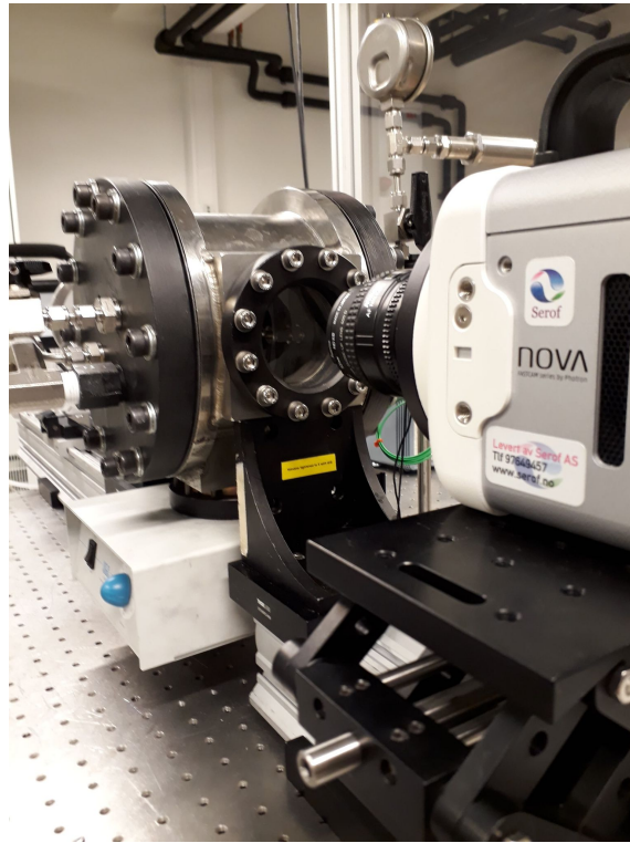
Side view of the high speed camera used during particle distribution analysis
