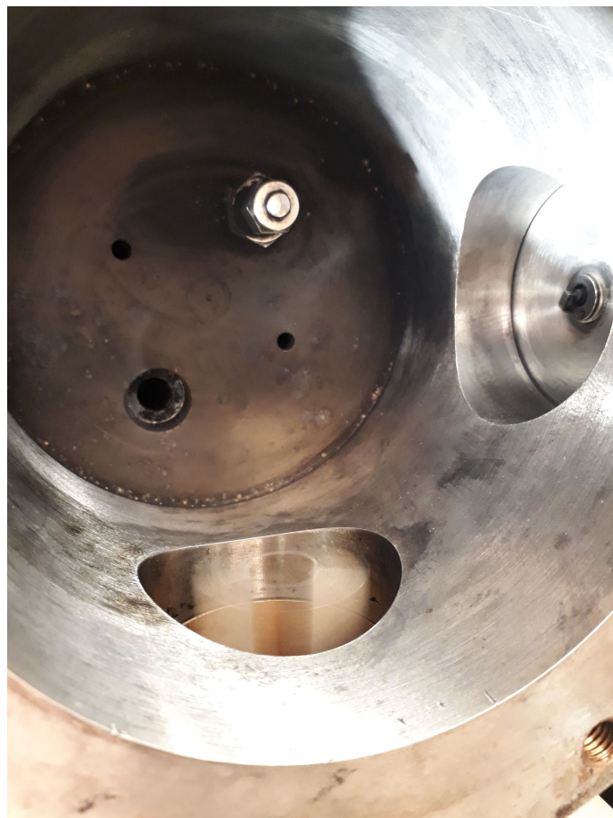
Inside the chamber with a rotating fan on the bottom, the spark-plug in the right pocket and gas injection pipes
