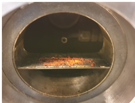
Figure 4.11: Typical result after static PI of CNTs particles within the chamber, 36 mg sample and Fe content of 66 wt%
