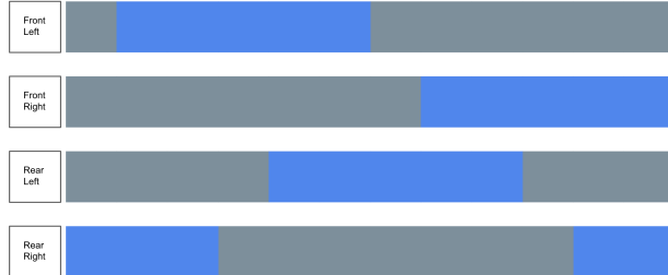
Figure 5.1: Diagram for one cycle of an ambling gait. Grey stretches indicate stance phases while blue stretches indicate swing phases.
