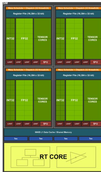
Figure 5.1: Turing architecture SM design. Used with permission from Nvidia.
