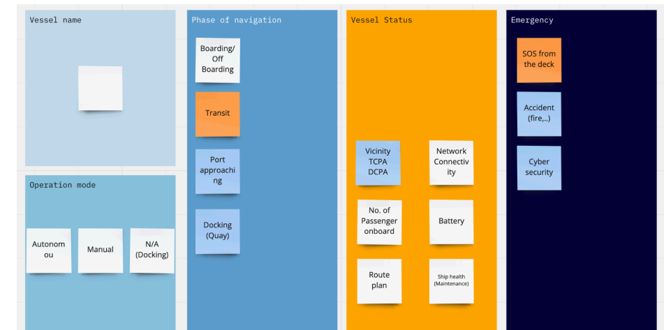
Figure 4.9 Components of the status panel
