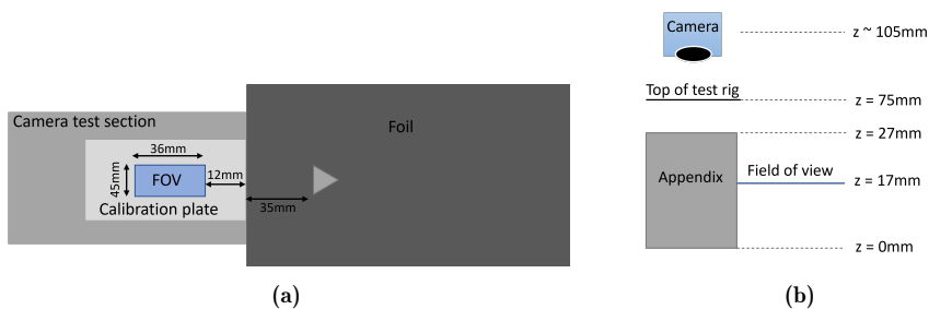
Figure 4.10: Description of the placement of the field of view in the a) xy-plane and b) zx-plane
